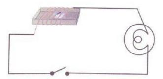
Ans: No. The given circuit does not have any current source. In the absence of current, the wire does not behave as a magnet and hence, the compass needle will not show any deflection.
