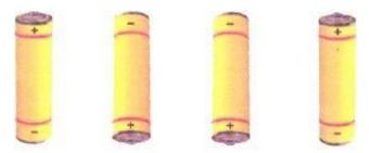
Ans: To make a battery, the negative terminal of one cell must be connected to the positive terminal of the next cell. The wire indicates the manner in which the given cells should be connected with each other, as shown in the following figure.
