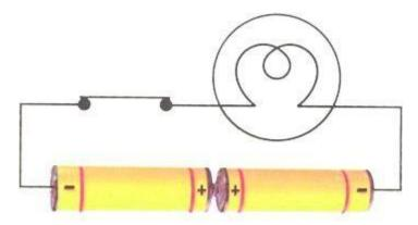
Ans: The bulb in the circuit is not glowing because the two cells are not connected properly.
